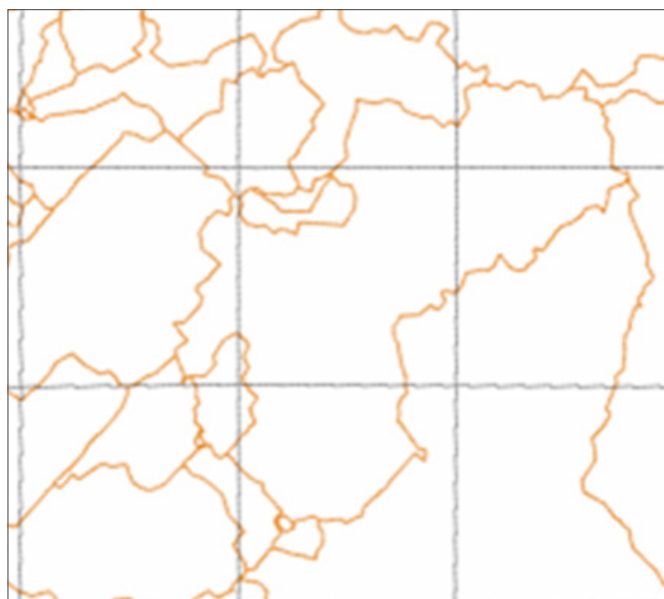
Figure 2-7. Example MODFLOW Grid (black) Overlain onto AHD Catchments (orange)
