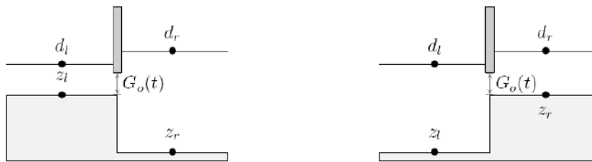
Figure 7.17 – Water levels for discharge under a gate in submerged conditions formulated as in (G1).
