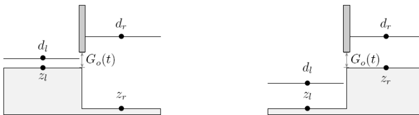
Figure 7.18 – Water levels for discharge under a gate in submerged conditions formulated as in (G2).
