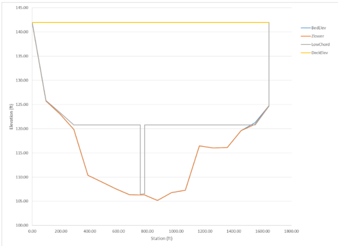
Figure 7.2 – Front view of a bridge cross section.
